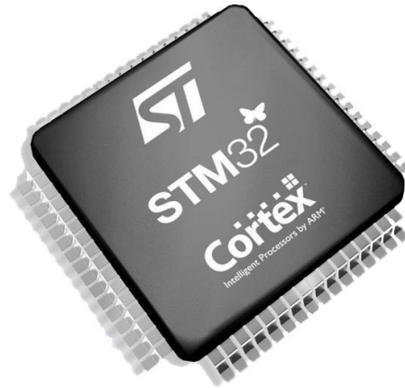
A 32-bit CORTEX microcontroller - with clock frequency 24 MHz, 8 kiB RAM and 64 kiB ROM (source: www.botland.com.pl )
