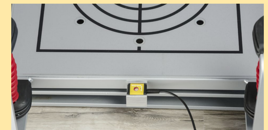
Fig.: Attaching the sensor, Posturomed® compact Alternatively: on the front outer frame of the standing platform
