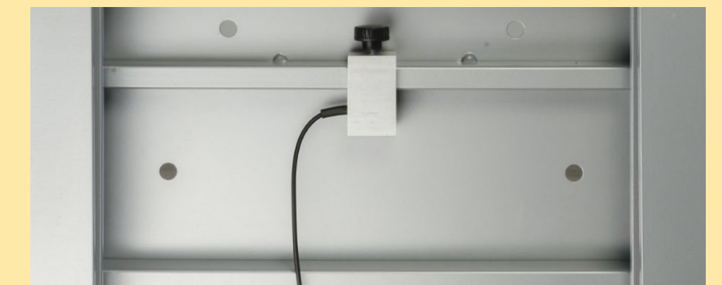
Fig.: Attaching the sensor, Posturomed® compact (underside) – Caution: configure the axis direction!
