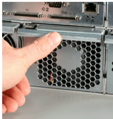
Figure 12. Replacing the cooling unit into the enclosure.
